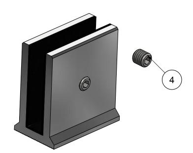
2x set screws included. 6mm glass use long screw 8-10mm glass use short screw
